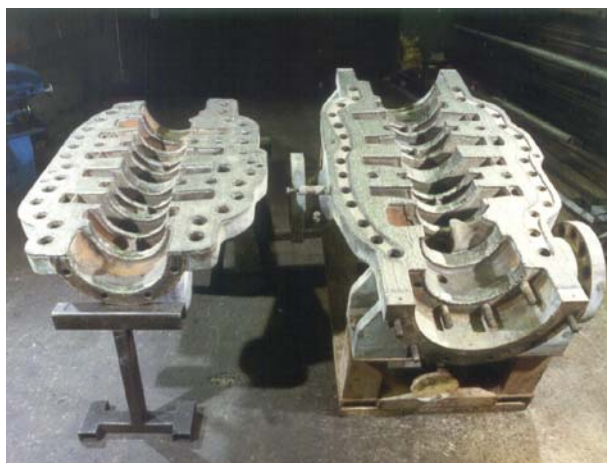
Pump casing after completion of the reclamation using Metrode Ultramet
