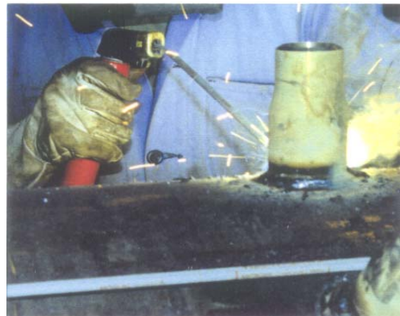
Welder using Chromet 9MV-N on fabrication of header
