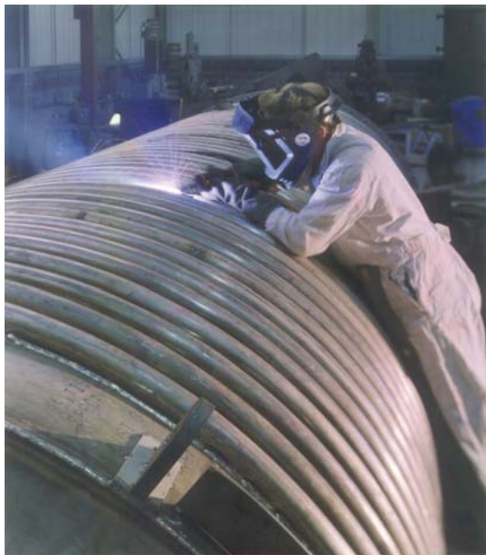
Welding of the limpet coil to the reactor vessel
